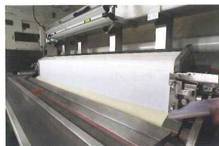
New Herma adhesives are made with the help of curtain coating technology
